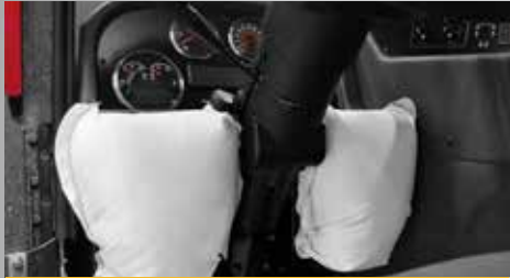
DRIVER KNEE AIRBAGS Protects the driver against contact injuries.
