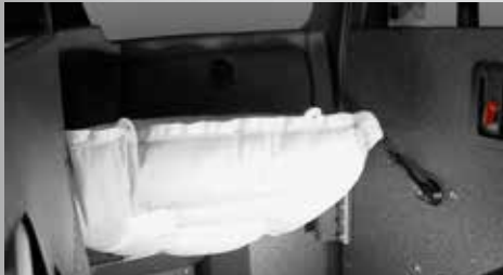
OFFICER KNEE AIRBAGS Protects the passenger from deceleration injuries.
