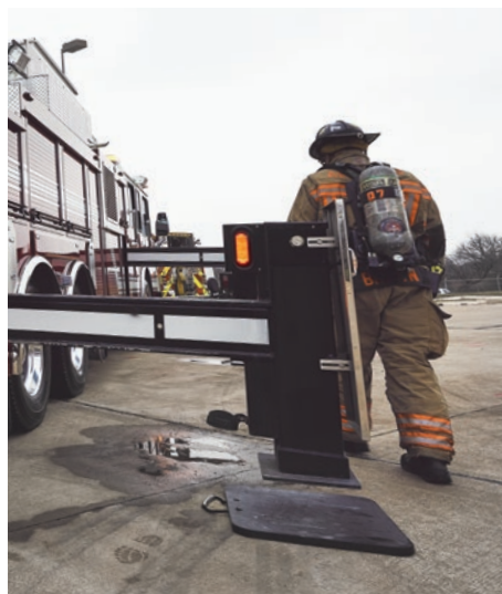
SPARTAN SELF-LEVELING SYSTEM (SSL): At the push of a button, after the outriggers are deployed the truck is automatically leveled. The optional SSL system also stows the outriggers at the touch of a button.
