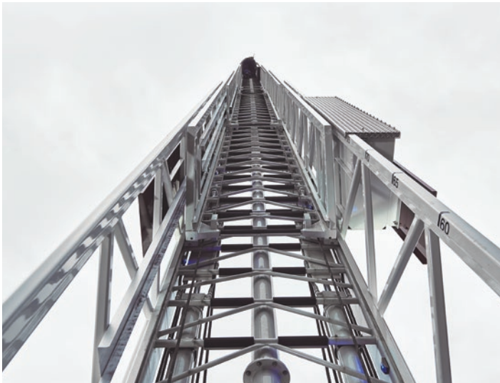
AERIAL LADDER DESIGN: All aerial ladder sections and primary load support members are designed with certified high-strength steel to ensure the highest quality with superior strength-to-weight ratios and minimal aerial ladder deflection.
