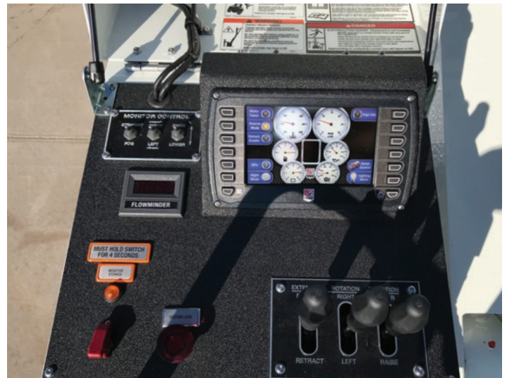
AL-11 AERIAL LOGIC: A totally integrated system that provides instant feedback on a ladder's extension, location, retraction, angle, load and breathing air system status, as well as J1939 engine information.
